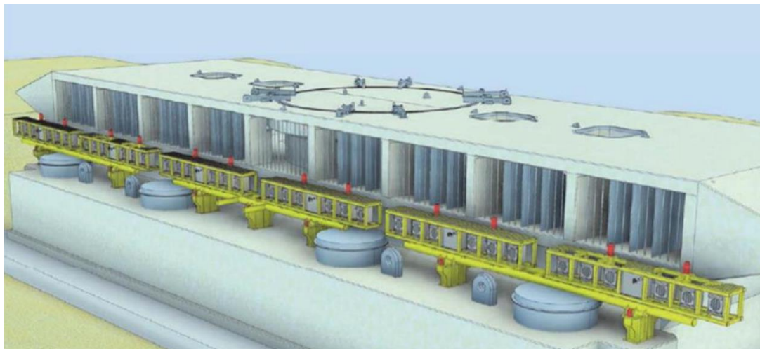
Figure 6.5: Preferred design for installation of sound projectors on an LVSE intake head
